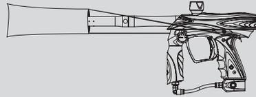
Screw the included barrel into the Epiphany. Put the supplied barrel blocker over the end of the barrel, securing its cord as far back on the Epiphany body as possible, and cinching it tight.
