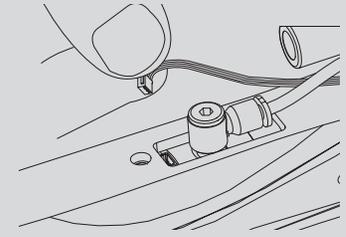
Locate the Vision wiring harness. This group of four black wires runs from the lower circuit board to the Vision circuit board in the body breach. Unplug the Vision wiring harness from the body end, being careful not to strain the wires by tugging on them. As much as possible, pull on the connector directly.
