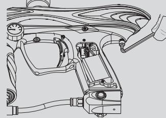
Remove the front and rear grip frame screws using a 5/32-inch allen wrench.
