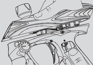
Grasp the body with one hand and the grip frame with the other. Slowly pull the body away from the grip frame, rolling it slightly to the side, exposing the top of the grip frame and banjo fitting. It can be helpful to gently push on the bottom of the circuit board with a thumb, helping it to slide upward.
