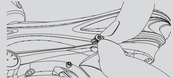
During normal maintenance the power button does not need to be and should not be removed. If it is damaged or requires replacement, grip it between a fingernail and thumbnail, and wiggle out, rear side first.
