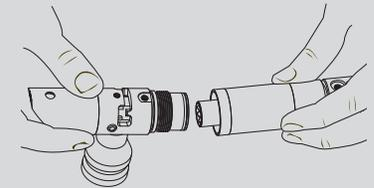
Unscrew the body breach from the fire chamber, and remove the bolt from inside. If the bolt stop does not come out with the bolt, pull it out with a finger.
