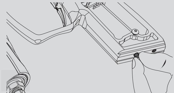
FIG. 8 → TIGHTENING SET SCREW
