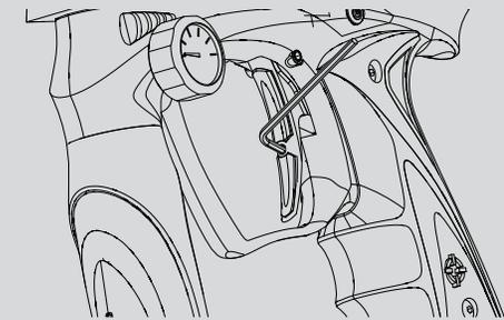
FIG. 15 → ADJUSTING ACTIVATION POINT
